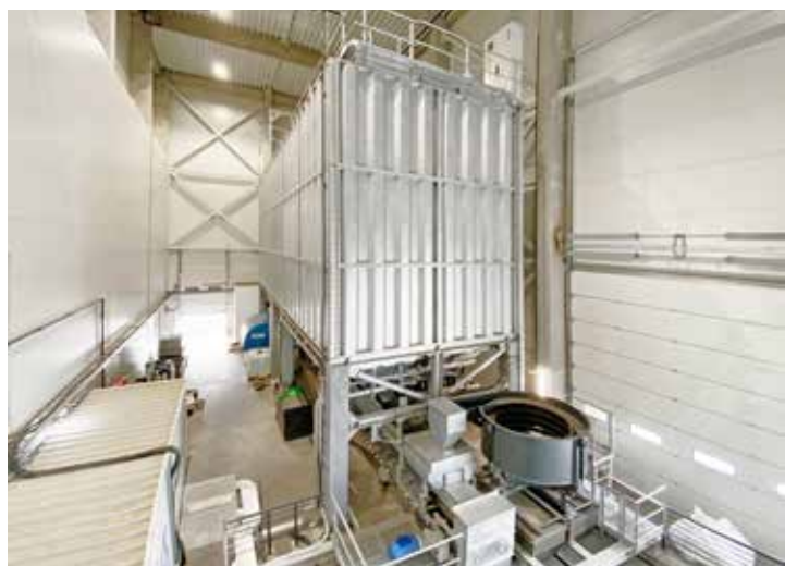
Massive aggregates storage and fiber dosing, all integrated in the production building
